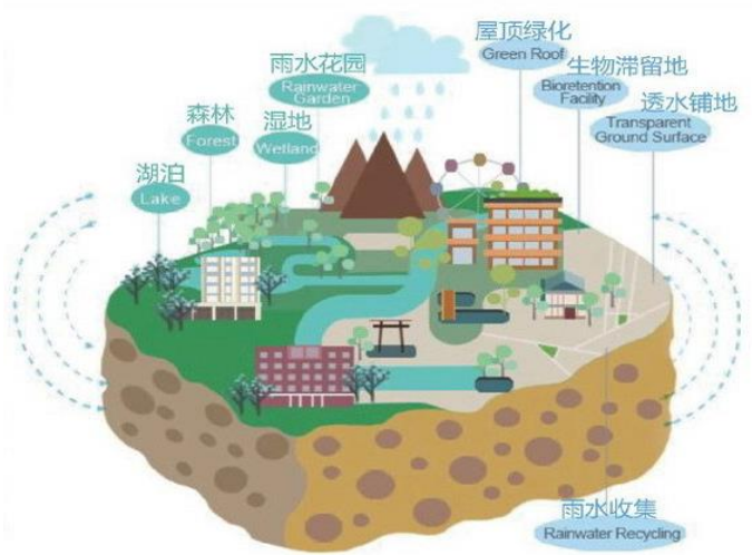
Fig.1 General Diagram of a Sponge City ( www.chinacitywater.org )
